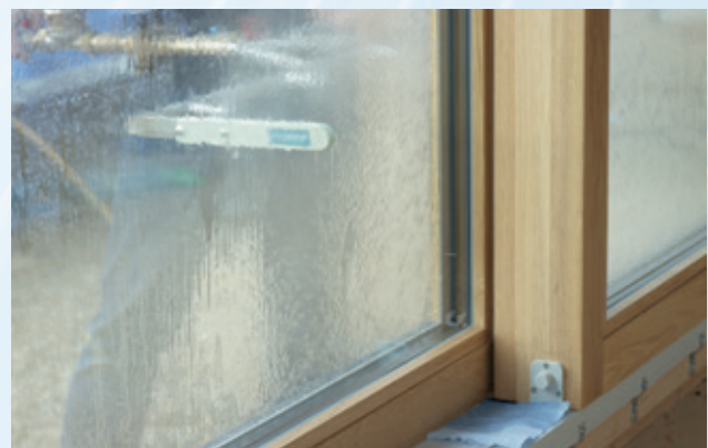
For optimal leakage detection, the SPRAY BAR is combined with the BlowerDoor measuring system
